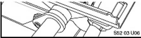
the end of the screw through the guide hole.
