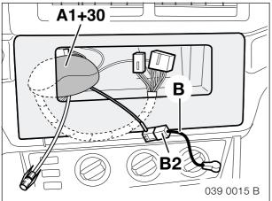
Lay the wrapped plug connector **A1** and new generation (30) on the left behind the instrument panel so as to enable you to install the navigation radio. ◀
