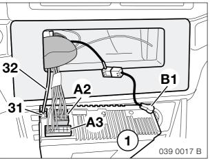
Connect branch **A2**, black 16-pin socket casing, to the navigation radio (1).
