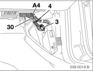
Carefully slide the connected navigation radio (1) into the radio shaft (30) and secure it with the existing slides.
