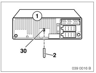
Screw the radio retaining pin (2) on to the stud bolt (30) on the navigation radio (1).
